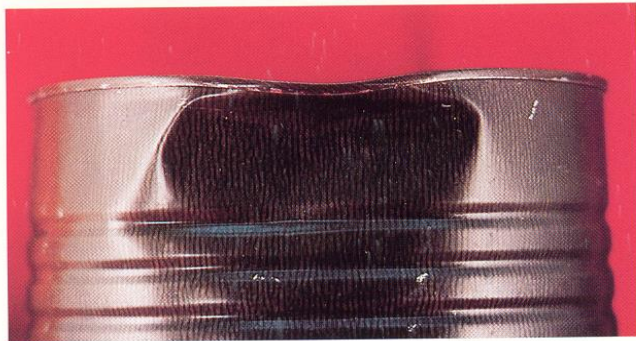
12. Major body dent which has impacted on double seam. (Plate may be fractured with loss of hermetic seal).
