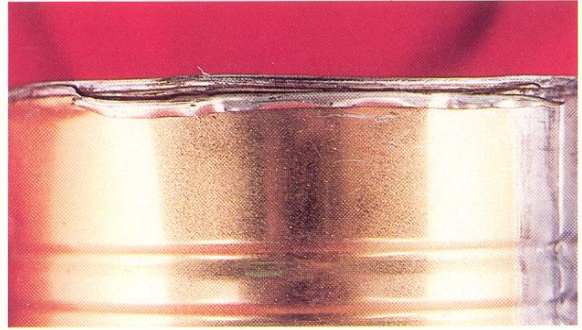
9. Depicts a false seam with loss of hermetic seal. Seam is formed but not engaged properly. (Note knocked down flange).
