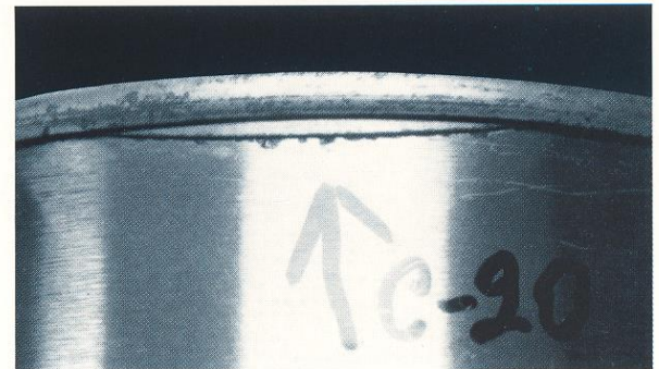
16. Pointer indicates "knocked down flange."
