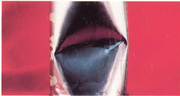
13. Major dent in center of can body. (Plate may be fractured with loss of hermetic seal).
