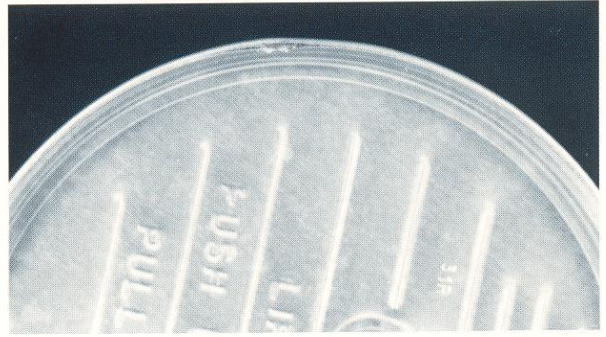
14. "Cut-over" depicting sharp seam. (Observe for potential plate fracture or loss of hermetic seal).
