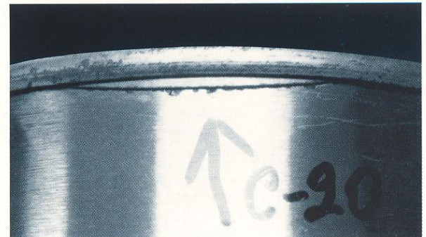
16. Pointer indicates "knocked down flange."
